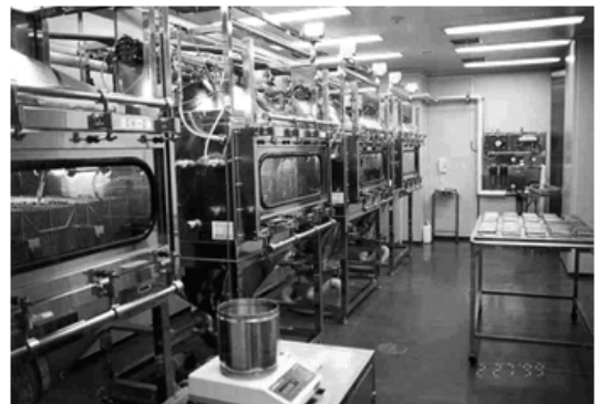
Photo 1. Exposure Inhalation chamber.
