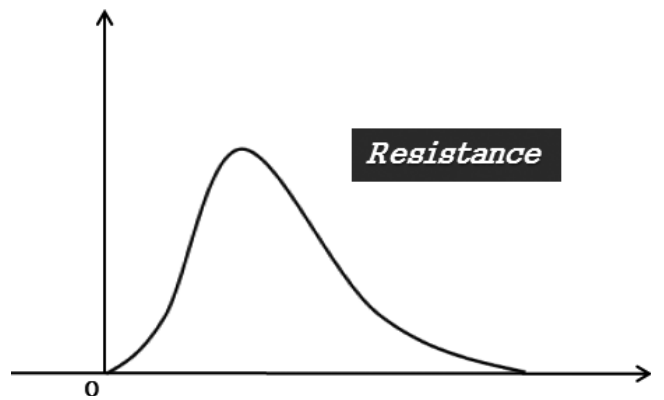
Fig. 3 Schema of the probability distribution of breaking strength
