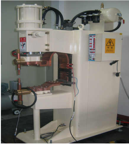
Fig. 2 Resistance spot welding machine(Compressed air type)
