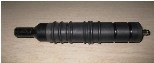
Photo. 2 Improved ultrasonic sensor for fuel pump
