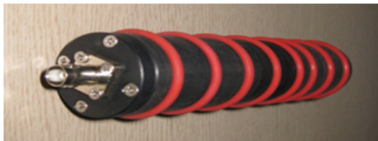
Photo. 3 Improved ultrasonic sensor for cylinder head
