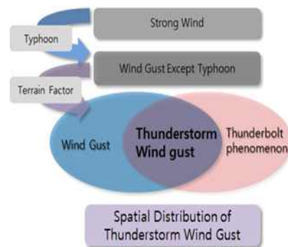
Figure 2. Classification Process of Thunderstorm Wind Gust from Wind Speed Records
