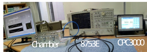
Fig. 6. Sensor characterization system. System is composed of vacuum chamber, network analyzer (HP 8753E) and precision pressure regulator (CPC3000)
