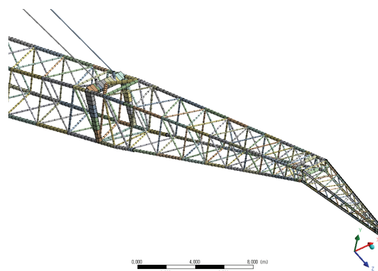
Fig. 3 Boom meshing result
