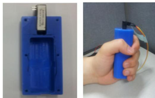
Figure 1. Structure of haptic handle and haptuator
