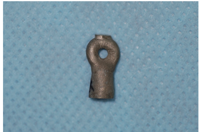
Fig. 3. Crown coping with a loop for retention testing.
