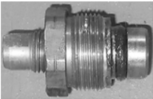
Fig. 8. Damaged O-ring in a valve stem.
