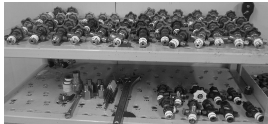
Fig. 3. Used valve samples for a leakage test pressure from 20 to 200bar.
