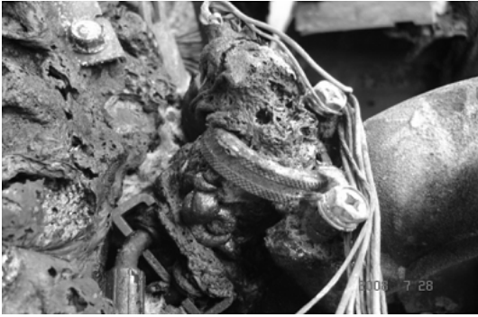
Fig. 8. Ring shape unseated from Number 4 injector.
