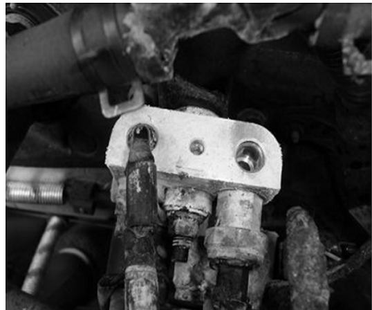
Fig. 4. LP gas connecting hose by fixing bracket.
