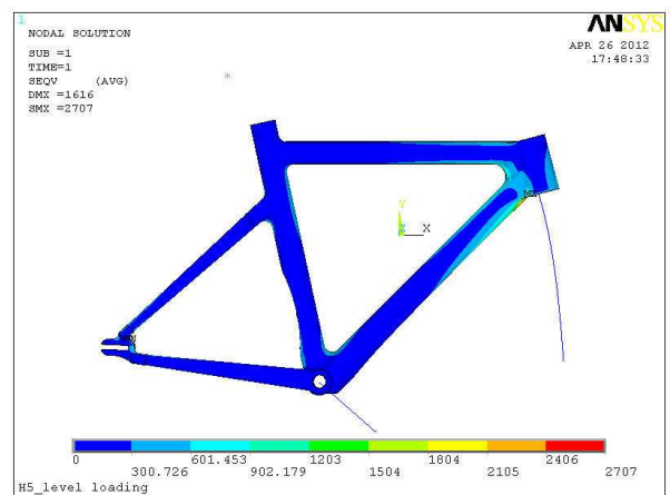
Fig. 12 Ha-frame von Mises stress results about level loading
