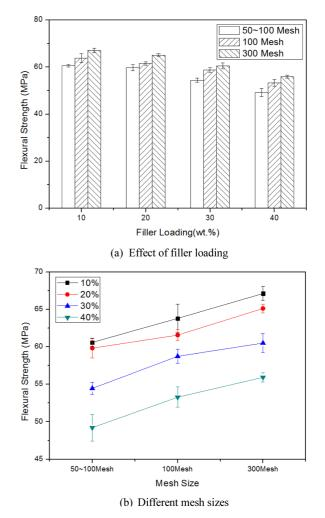
Fig. 1. Flexural strength of the CHF/PP Composites.
