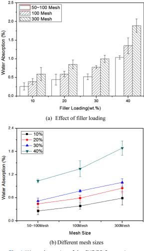
Fig. 4. Water absorption of the CHF/PP Composites.
