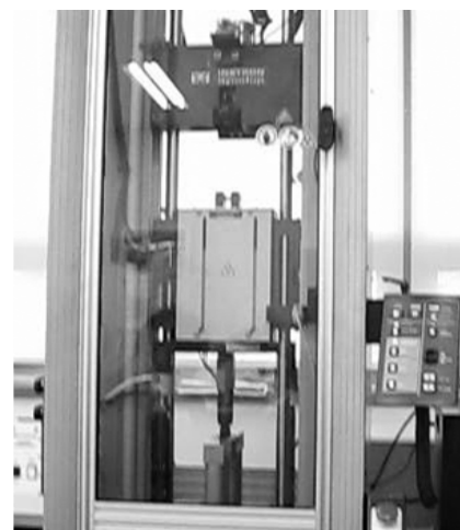
Fig. 1 (a) Geometry of impact test specimen (unit : mm), (b) Drop weight impact tester (Instron 9250Hv) (unit : mm)
