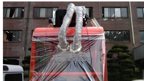
Fig. 6 The blow motor and exhaust pipe
