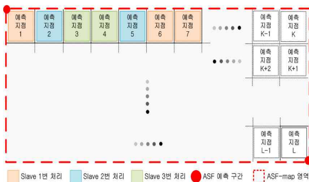
Fig. 4 Parallel processing of ASF simulator in Slave part
