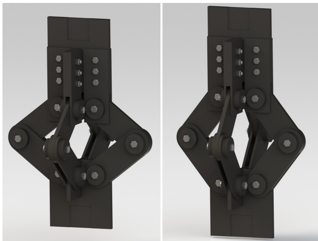
Fig. 5. Configuration of rotational friction damper
