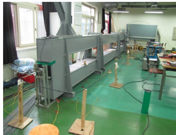
Fig. 5. Tensile stress testing machine and closed loop magnetic circuit
