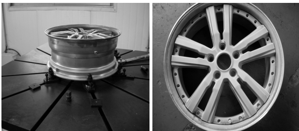
Fig. 12 Cornering fatigue test and penetrating tests
