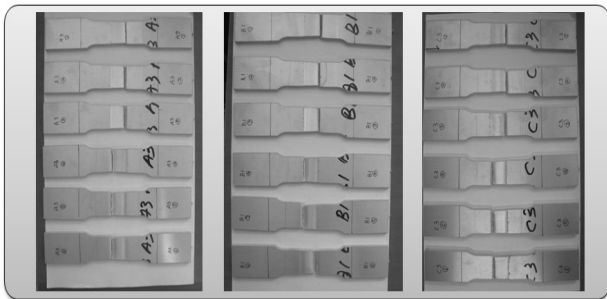
Fig. 4 Tensile specimen produced by FSW
