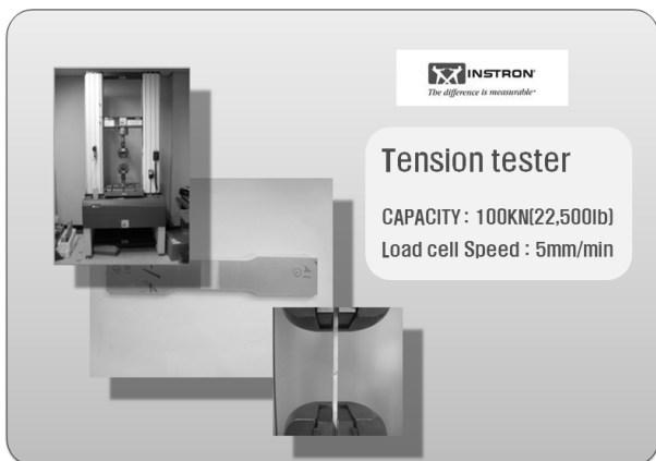
Fig. 5 Tensile machine used in this work
