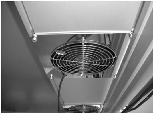
(c) ASU assembled under the air bed (table)
