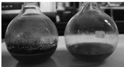
Fig. 1. Comparison of effect of solvent on extraction efficiency between methanol (left) and 95% ethanol (right).
