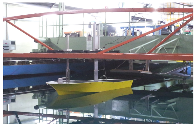
Fig. 3 Setup for model tests of a 40ft class leisure boat
