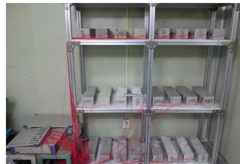
Figure 1. Drying shrinkage test
