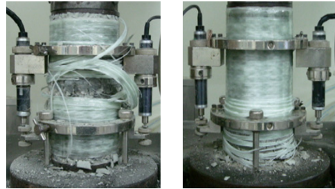
[Fig. 10] Failure mode of specimen
