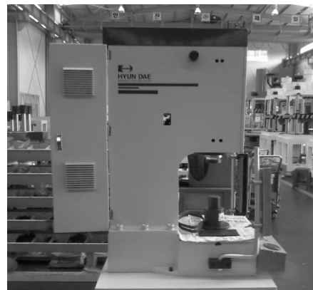
[Fig. 2] Test model of servo-press type pressing machine
