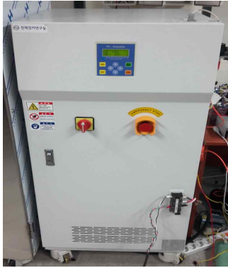
Fig. 26 The PV simulator
