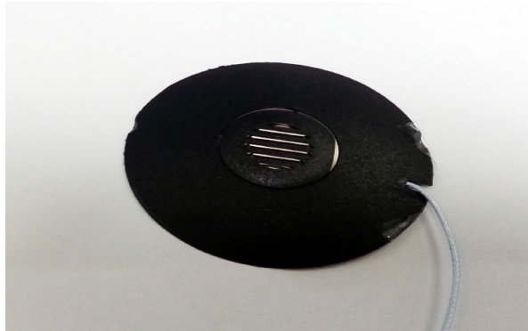
Fig. 2 Patch Type Microphone (B&K, Type 4949)
