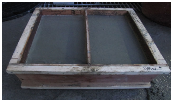
(a) Existing PCC for Pull-Out Test (500×250×150mm)
