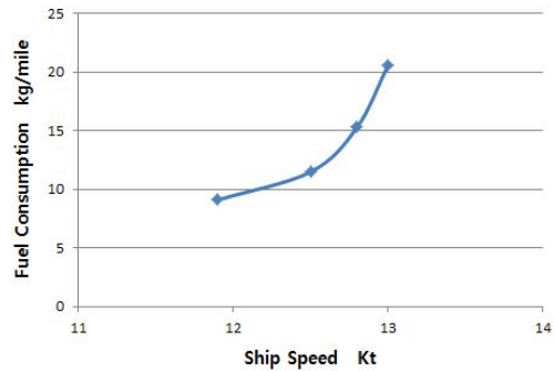
[Fig. 3] Relation between ship speed and fuel consumption
