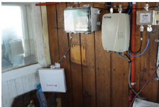
[Fig. 2] Photograph of TRS system installed in the trial fishing boat
