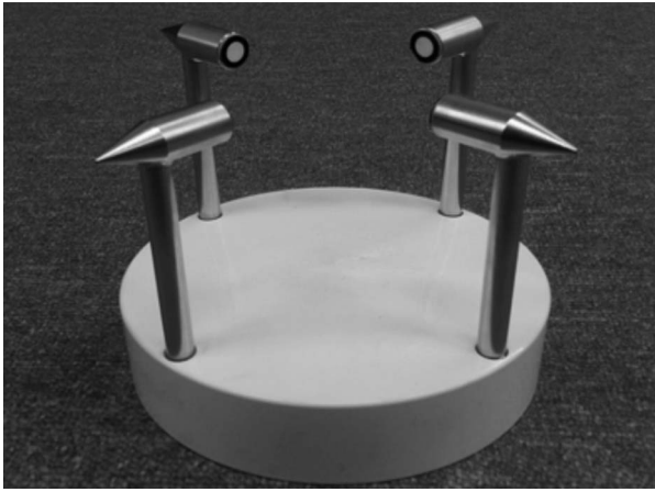
Fig. 3. Trial manufactured wind sensor.
