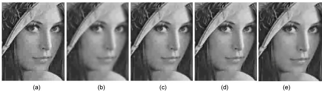
그림 4. Lena 영상에 대한 주관적 화질 비교 (a) JPEG 압축 영상(0.25bpp; PSNR = 30.40dB), (b) Zakhor 방법(29.03dB), (c) Chen 방법(31.22dB), (d) DFOVS 방법(31.01dB), (e) 제안한 방법(31.34dB) Fig. 4 Comparison of subjective quality for Lena (a) JPEG-compressed image (0.25bpp; PSNR = 30.40dB), (b) Zakhor's method (29.03dB), (c) Chen's method (31.22dB), (d) DFOVS (31.01dB), (e) proposed method (31.34dB)
