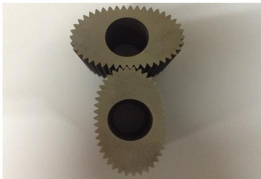
**Fig. 15** Manufactured oval gear set by WEDM designed for  $m=0.6$ , pressure angle= $30^\circ$ , teeth=42
