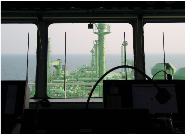
Fig. 1. Interference with watchers' vision under sail at the bridge of H. No.2258 built in DSME shipyard.
