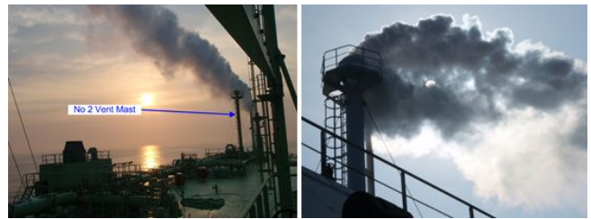
Fig. 5. Photo of LNG gas dispersion during gas trial.
