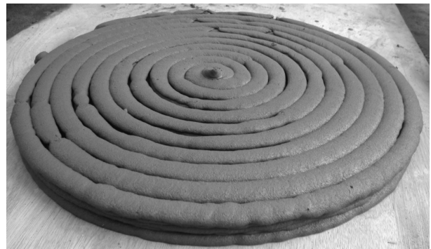
Fig. 15. Spiral structure construction using Automated Freeform construction system
