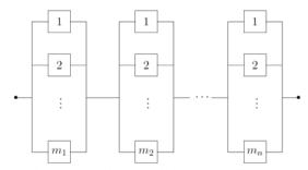
Figure 1. Series-parallel system diagram
