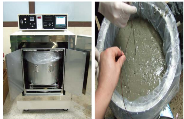
Fig. 3 Adiabatic Temperature rise tester
