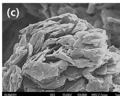
Fig. 2. Scanning electron microscope images of raw graphite powder (a), graphite powder mixed with coal tar pitch (b) and graphite powder mixed with phenolic resin (c).
