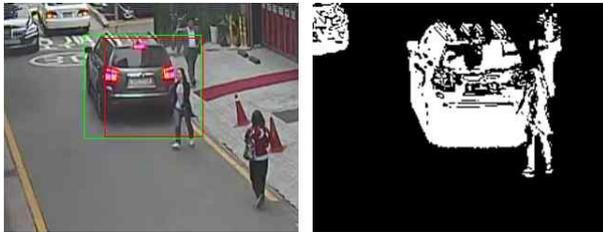
Figure 7. An Example of Object Overlapping (Left) and the Corresponding Background Subtraction Result (Right)
