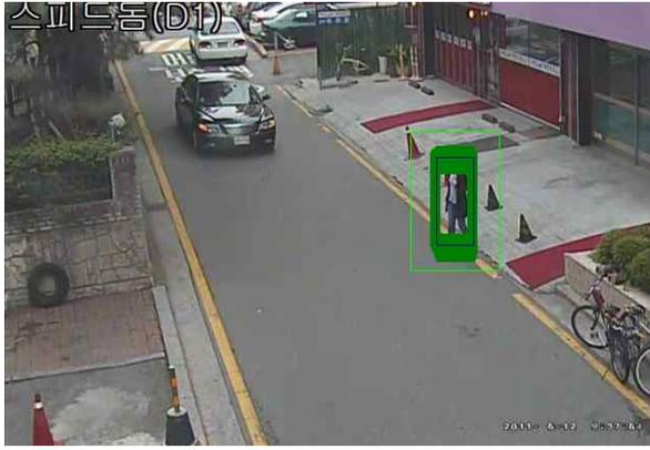
Figure 6. Detected Object Location (Black Box) and Object Location with High Matching Rate (Above 10% of Matching Rate, Green Region)
