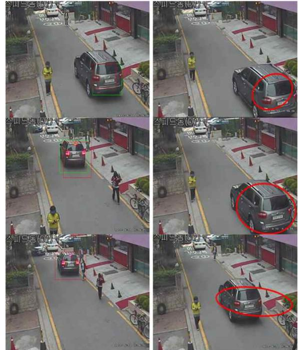
Figure 9. Vehicle Tracking Results of Proposed Approach (Left) and CamShift (Right)
