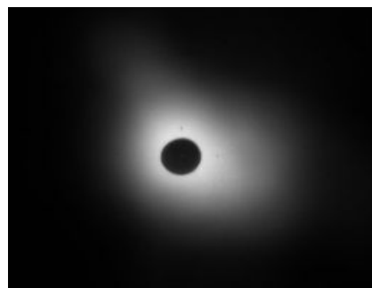
Fig. 7 Diffuse target surface image at the 5 kW KIER solar furnace
