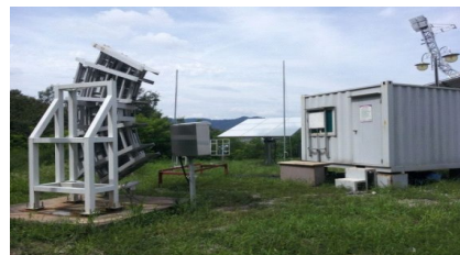
Fig. 6 Picture of the 5 kW KIER solar furnace
