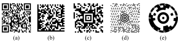
그림 4. 2차원 바코드의 종류 : (a) QR Code, (b) Data Matrix, (c) Aztec code, (d) Maxi code, (e) Shot code Fig. 4. 2-D barcodes : (a) QR Code, (b) Data Matrix, (c) Aztec code, (d) Maxi code, (e) Shot code
