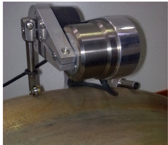
Fig. 1 An image of Miniprof device implemented on a wheel
