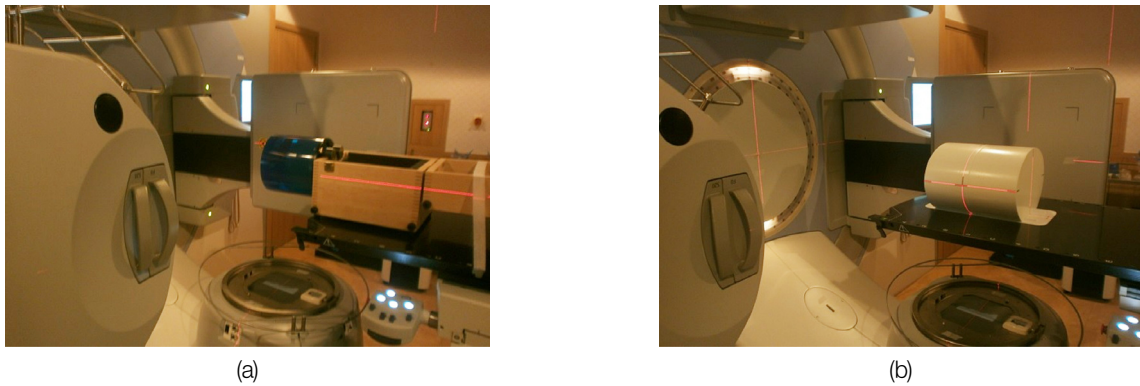
Fig. 3. The setup of phantoms for 3D image acquisition (a) Catphan503 phantom, (b) Homogeneous phantom
