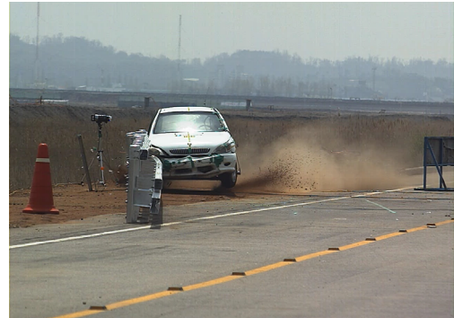
[Fig. 9] Full-scale crash test using the small car impact speed of 130km/h
