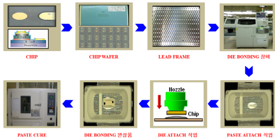
[Fig. 1] Typical die bonding process for LED chip fabrication.
