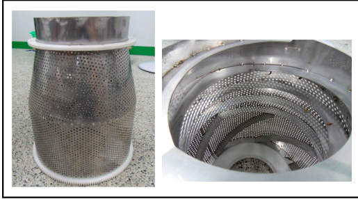
Fig. 2. Drum and spiral blade of washer for boxthorn berries
