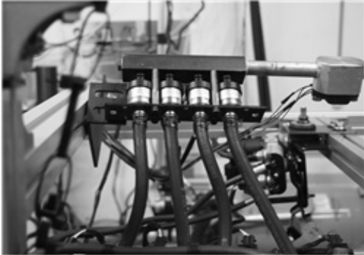
Fig. 2 Gas injector installation in the intake system
