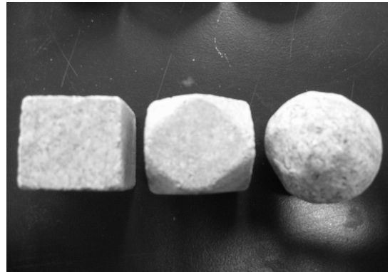
Fig. 7. Shape of rock lump used in slake durability test (From left; Hexagonal, Hexagonal with rounded corner, Spherical)
