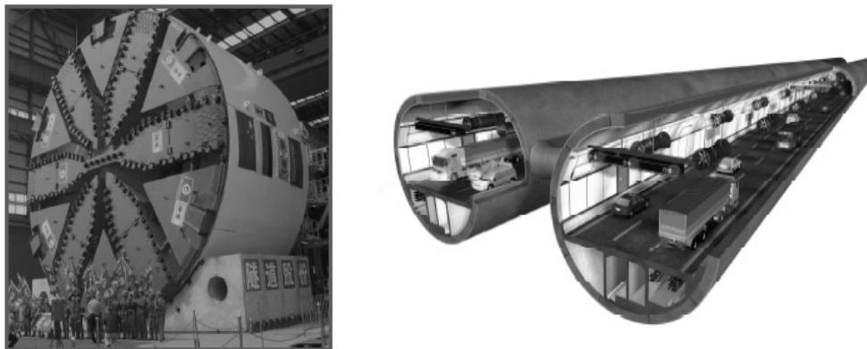
Fig. 2. World's large scale soft-ground TBM for Xangxing tunnel, Shanghai, China
