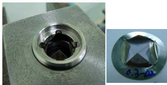
Fig. 7. Nozzle closure shape after bursting
