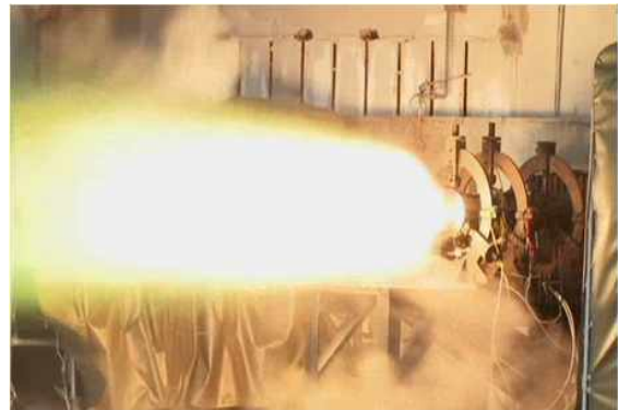
Fig. 10. Static fire test to evaluate a gas gen-erator
